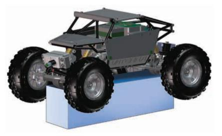
Perform a control test with the vehicle wheels off the ground. If the wheels rotate after the vehicle is powered ON, adjust the "TH. Trim" knob until they stop. To make the wheels move forward, pull the trigger. To reverse them, wait for the wheels to stop, then push the trigger. When moving forward, the wheels should maintain a straight line without any steering wheel input. If not, adjust the "ST. Trim" knob so the wheels maintain a straight line without having to turn the steering wheel.
