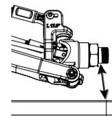
To reduce droop (higher measurement number), turn the droop screw for the suspension arm clockwise. To increase droop (lower measurement number) turn the droop screw for the suspension arm counterclockwise. After making an adjustment, compress the suspension by hand, then allow it to settle before measuring again.
