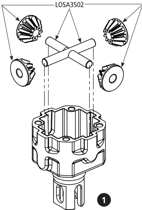
**EN** Fill with 7000 wt oil to a weight of 43.2g. Use a scale accurate to .01g
