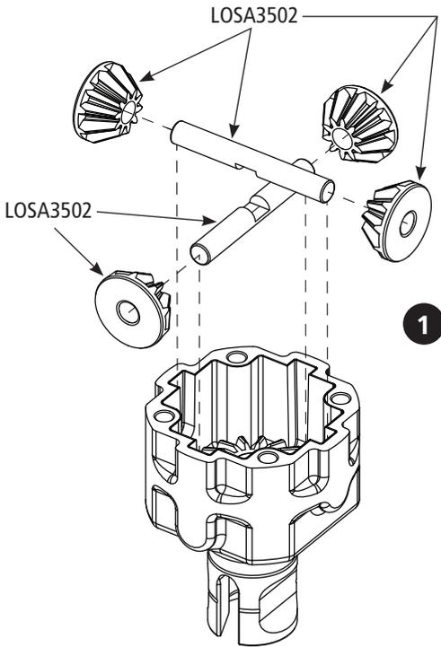
**EN** Fill with 4000 wt oil to a weight of 42.7g. Use a scale accurate to .01g
