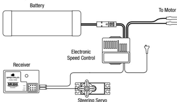
3. With the steering wheel, throttle trigger and Aux channel (if applicable) in the desired preset failsafe positions (generally full brake and neutral steering), initiate the bind process with your Spektrum transmitter. This stores the failsafe positions. Continue to hold the failsafe positions until the binding process is complete. Please see the next section for more information about failsafe.
