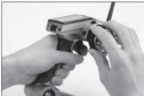
4. Follow the procedures of your specific transmitter to enter bind mode; the system connects within a few seconds. Once connected, the LED on the receiver will go solid indicating the system is connected.
