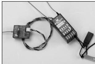
2. Power the receiver. The LED on the receiver should be flashing, indicating that the receiver is in bind mode and ready to be bound to the transmitter.
