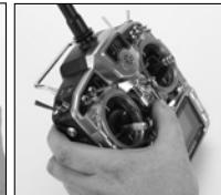
4. Follow the procedures of your specific transmitter to enter Bind Mode, the system will connect within a few seconds. Once connected, the LED on the receiver will go solid indicating the system is connected.
