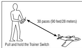
1. With the model restrained on the ground, stand 30 paces (approx. 90 feet/28 meters) away from the model.
