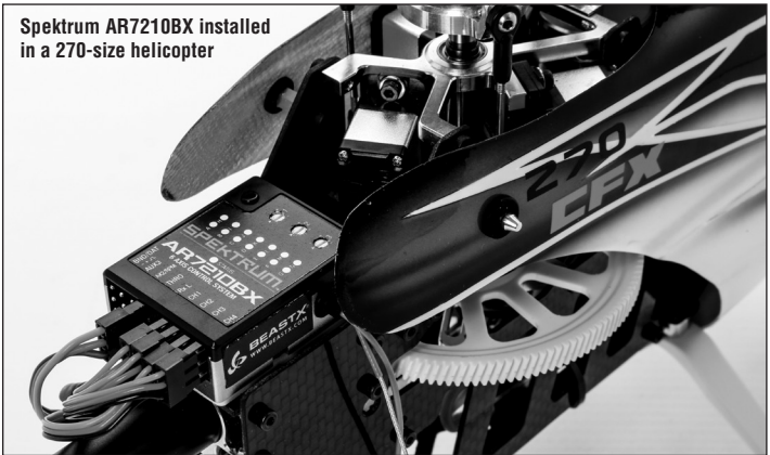
Spektrum AR7210BX installed in a 90-size helicopter with remote receiver
