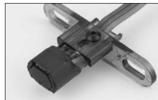
Bracket adjusted for 90-size engine
