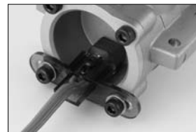
Bracket adjusted for 90-size engine
