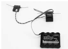
Shown using a separate receiver pack. (Battery can be plugged into any open port.)
