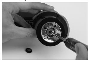
**Note:** Proper alignment of the steering wheel with the steering wheel mechanism stops should be observed for correct reassembly.
