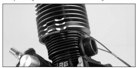
Plug the temperature sensor into the port marked E in the telemetry module. The handheld unit should now display room temperature.
