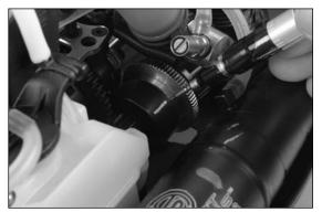
Set the car next to a ruler and at 0" then roll the car forward by hand, counting each revolution of the reference mark. At exactly 10 revolutions stop the car.
