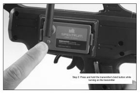
It is necessary to bind the handheld unit to the transmitter. Binding teaches the handheld unit the specific code of the transmitter and when bound, the handheld unit will only listen to information coming from the receiver(s) that are bound to that transmitter. To bind the handheld unit:
