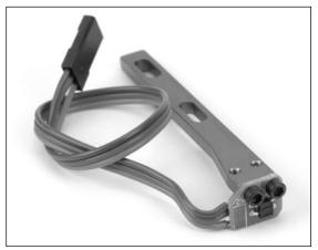
Install the mount under the engine screw and adjust the sensor so it is 1/8" from the flywheel.
