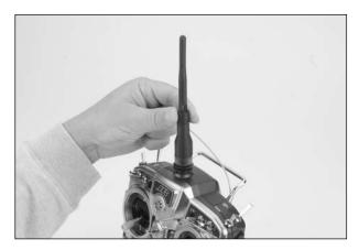
Carefully install the Spektrum module into the transmitter paying close attention to properly align the pins.
