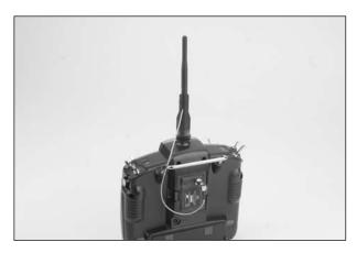
5. Turn on your transmitter. The LED on the back of the module should come on after a few seconds. If not check to be sure the transmitter is in PPM modulation mode (Step 3 in preparing the transmitter above).
