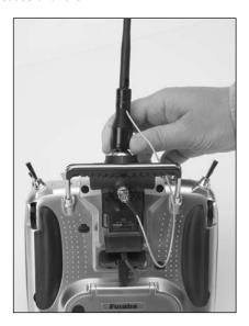
Place the transmitter in PPM mode. This is done in the modulation menu in your transmitter's programming. See your Futaba MZ radio manual for specific details if necessary.
