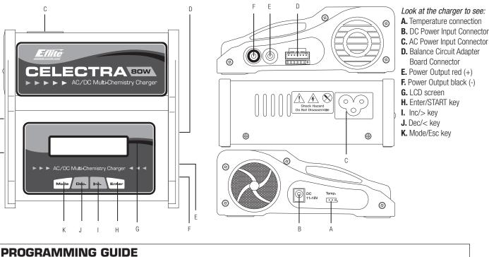
Press the Mode key (K) to change among main menu screens or to get to these main menu screens from a submenu screen. Press the Enter key (H) to get to submenus for adjusting operating parameters, to save value changes, or to start chosen battery charging actions. Press the Dec (J) or Inc (I) keys to change between submenu screens or to change (Decrease or Increase) screen values.
