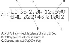
E. Present charge level of the battery is 1082mAh **F.** Time elapsed since the charge process started is 22:43 (22 minutes and 43 seconds) During charging, the Dec key can be pressed to show several
