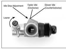
High-Speed Needle: 4 turns out (counterclockwise) from closed
