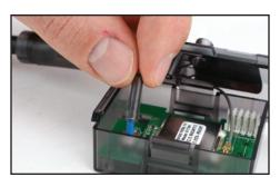
10. Put four screws in case bottom and screw case back together. **WARNING:** Be sure the antenna wire is not crimped between the cases. Do not over-tighten the screws or the case could be damaged.
