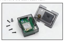
4. Remove the antenna wire by lifting up on it close to where it connects to the circuit board.
