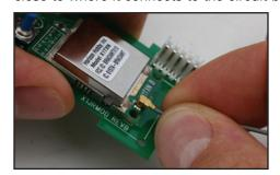
5. Connect the antenna of the new case top to the circuit board. Align the antenna with the connector on the circuit board. Apply a light pressure to the top of the antenna connector and it will pop into place.
