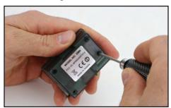
3. Remove circuit board from the bottom case.
