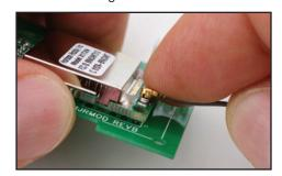
6. Swivel the antenna connector back and forth. If connected correctly, the antenna will swivel freely. If it doesn't, the antenna is not connected correctly. If the antenna is not connected correctly, remove the antenna and inspect the connectors for damage. If you think they are damaged, please contact product support (contact information is listed at the end of the manual).
