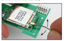
7. Place circuit board in the new case bottom. Be sure the white connector is aligned over the holes in the case bottom.
